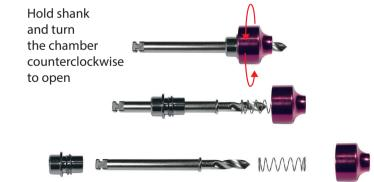
For cleaning and sterilization note that the chamber needs to be unscrewed, exposing the drill, hub and spring. For a total four (4) individual parts. Guide Pins are monoblocks and connot be disassembled.
